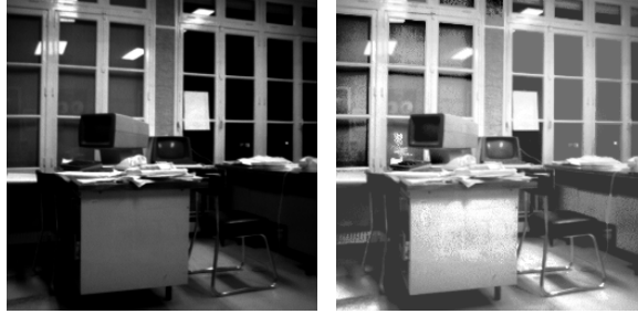
figure 7.2. Example of contrast enhancement. Note how objects that are not visible on the original image on the left (e.g., the 2nd chair and the objects through the window), are now detectable in the processed one (right).
