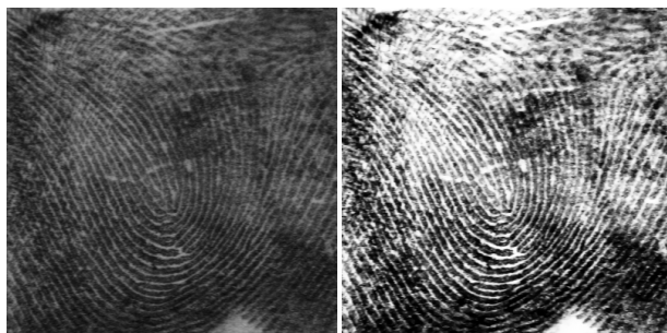
figure 7.5. Result (right) of simultaneous histogram equalization and anisotropic diffusion for a fingerprint image (left).
