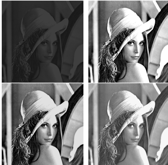
figure 7.3. Original image (top-left) and results of the histogram equalization process with the software package xv (top-right), the proposed image flow for histogram equalization (bottom-left), and the histogram modification flow for a piece-wise linear distribution (bottom-right).
