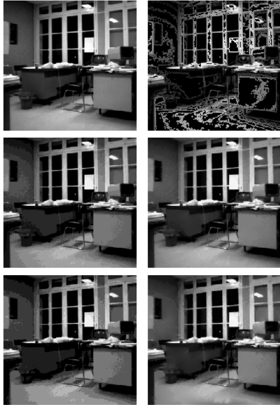
figure 8.1. Interpolation via PDE's. From left to right, top to bottom: Original image, level lines for \delta = 30 , quantized image for \delta = 20 , the interpolant for \delta = 20 , quantized image for \delta = 30 , the interpolant for \delta = 30 .
