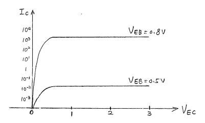
Where A=1 and  $D=0.026 \times 300 = 7.8$   $L=0.026 \times 300 = 7.8$   $L=0.88 \times 10^{-3}$  cm.  $T_B=5 \times 10^{-7}$   $W=0.32 \times 10^{-4}$  cm.  $N_B=5 \times 10^{16}$  cm<sup>-3</sup>  $N_E=2 \times 10^{17}$  cm<sup>-3</sup>
