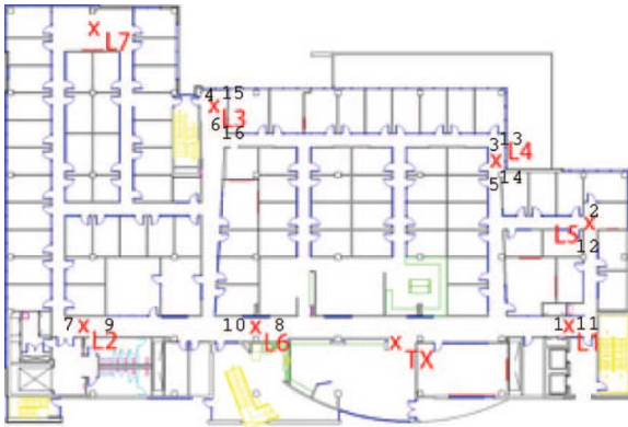
Fig. 3. 2nd Floor of ECERF: Indoor office measurement scenario from http://www.ece.ualberta.ca/~mimo/ .
