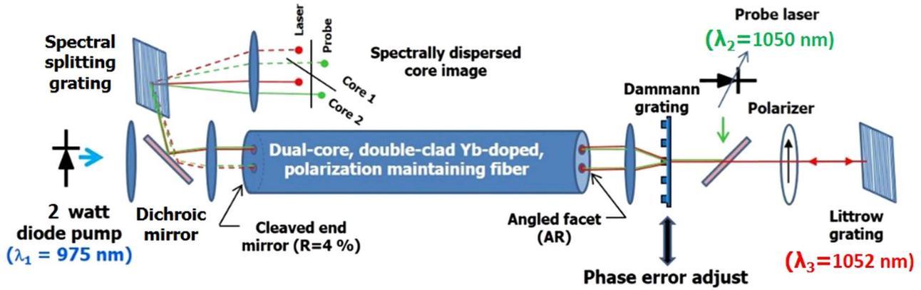
Fig. 2. Experimental configuration of the passively coupled laser cavity with associated diagnostic instrumentation.
