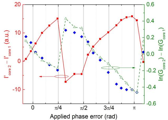
Fig. 5. Difference of the optical output intensities in the two gain arms (red solid squares) and the corresponding difference in exponential gain (blue solid diamonds) measured as a function of the applied phase error. The calculated difference in exponential gain (green open triangles) is obtained by using the experimental data of the output powers (red solid squares in this graph) along with the gain saturation results of Fig. 4.
