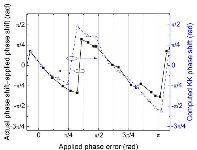
Fig. 6. Experimentally observed self-phasing (black solid squares) and the computed KK phase shift (blue open triangles) plotted as a function of the applied phase error. The computed KK phase shifts are inferred from the applied phase error versus output intensity data in Fig. 5, the output intensity versus gain relationship in Fig. 4, and the gain versus phase relationship in Fig. 3.
