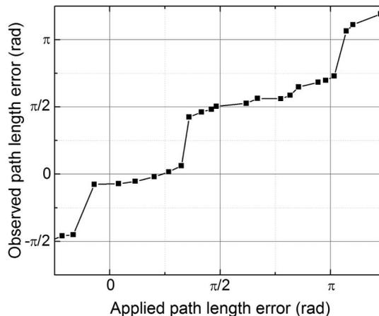
Fig. 1. Experimental data showing self-phasing in the passively coupled laser cavity. The height between the two adjacent phase steps is roughly equal to  $\pi/2$ .
