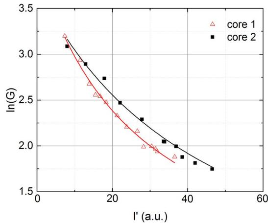
Fig. 4. Small-signal exponential gain versus the optical output intensity  $I'$  in each individual fiber core.
