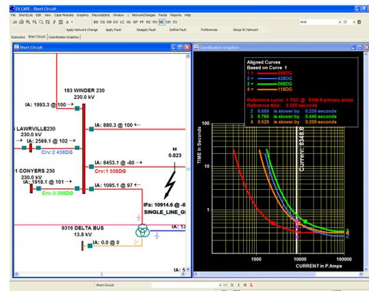
CAPE can display the complex characteristics of all types of distance protection. Above, you can drag a fault to see instantly how coordination time intervals change.
