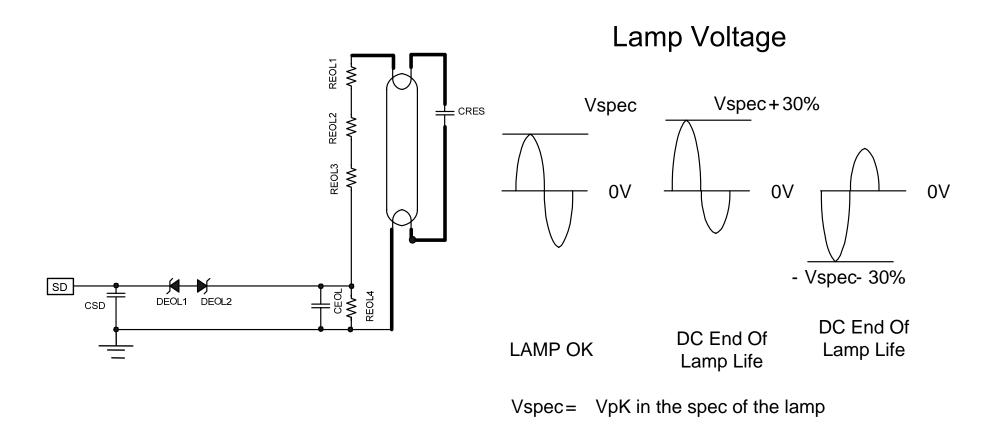
The SD pin is internally biased at 2V. During end of life the lamp voltage will increase asymmetrically (DC end of life). The voltage offset sensed at the top of REOL4 will increase and one of the Zeners will turn on, therefore triggering the shutdown.
