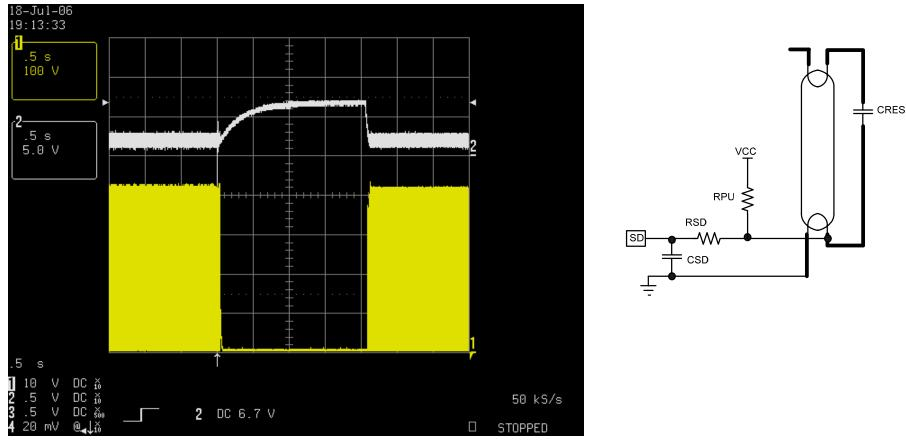
SD pin (upper) and half-bridge voltage (lower) during lamp out/re-insert condition **I**
