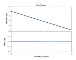
Solutions to Q. 2: The phase of the plant is constant at -180. Thus to have a phase margin of 45° the controller needs to have a phase of 45° at gain crossover. We will choose the gain crossover frequency  $\omega_c = \omega_m$  where  $\omega_m = \frac{1}{T\sqrt{\alpha}}$  where the lead controller has the maximum phase. Thus we need  $\phi_m := \angle \{G_c(j\omega_m)\} = \pi/4$ . This implies that
