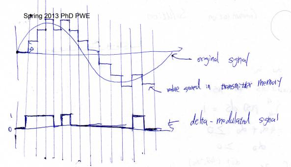
To avoid slope overloading, we need the signal value change in adjacent-
