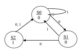
(c) Use two least significant bits of the counter  $q_1q_2$  to encode 3 states. From the transition diagram: transitions  $S0 \rightarrow S1$  and  $S1 \rightarrow S2$  can be implemented via counting function. All other transitions (to state S0  $\sim$  00) are implemented using CLEAR function. So, we use this state assignment S0~00, S1~01, S2~10. Count up function requires Load=0, Count=1.Clear input should be zero whenever input R=1 or when the system is in state  $S2(q_1=1)$ . Hence,
