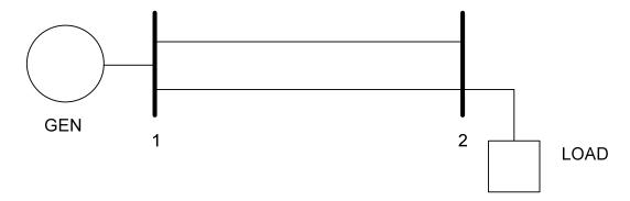
The load at bus 2 draws 5.0 pu MW and 0 pu MVAR from bus 2
