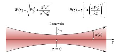
Here  $\lambda$  is the wavelength and  $W_0$  is the beam radius at the center.
