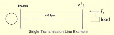
We assume that the voltage at the sending end is 1.0 per unit at zero degrees phase angle, and where *Qload* is assumed to be zero MVAR.
