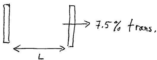
a) Saturated gain must balance loss in cavity
