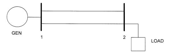
The load at bus 2 draws 2.5 pu MW and 0 pu MVAR from bus 2
