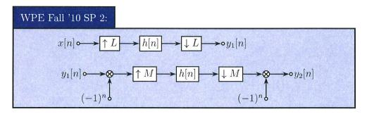
The digital filter prototype, with impulse response h[n], was designed to meet the following specifications
