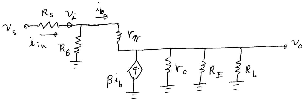
For  $R_{in}$ : Let  $R_L' = R_L \parallel r_o \parallel R_E = 794 \Omega$
