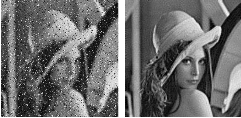
FIG. 2.1. Image deblurring in the presence of salt and pepper noise. Left: Source image blurred by a pill-box kernel of radius 3, and contaminated by noise of density 0.1. Right: Recovered image using the algorithm analyzed in this paper.
