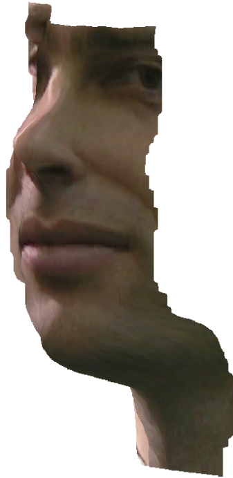
figure 3.30. 3D reconstruction from a stereo pair using the geodesic stereo approach. First, the stereo pair is shown, followed by the reconstructed 3D shape.
