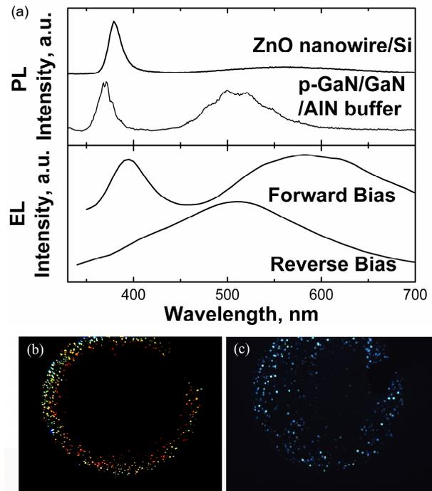
**Figure 2:** (a) PL spectra of ZnO nanowire arrays and p-GaN film and EL spectra of ZnO nanowire/p-GaN film heterojunction, (b) and (c) top view image (100x) micrograph of EL emission under forward and reverse bias, respectively.
