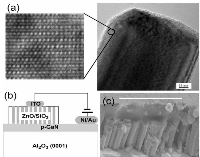
**Figure 1:** (a) High crystallinity evidenced by high resolution TEM, (b) heterojunction device structure, and (c) SEM image of ZnO nanowire array surrounded by SiO<sub>2</sub> on p-GaN, scale bar: 5  $\mu\text{m}$
