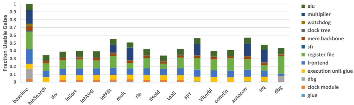
**Figure 10: The height of a bar represents the fraction of gates that can be toggled by a benchmark. Components within each bar represent each module’s contribution to the fraction of gates toggled by the benchmark.**
