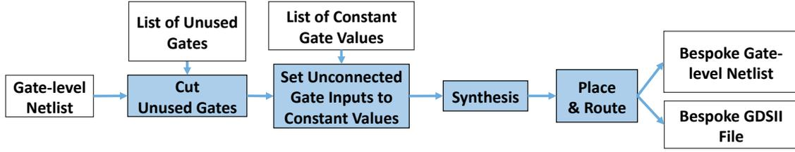
Figure 6: Tool flow for cutting and stitching.
