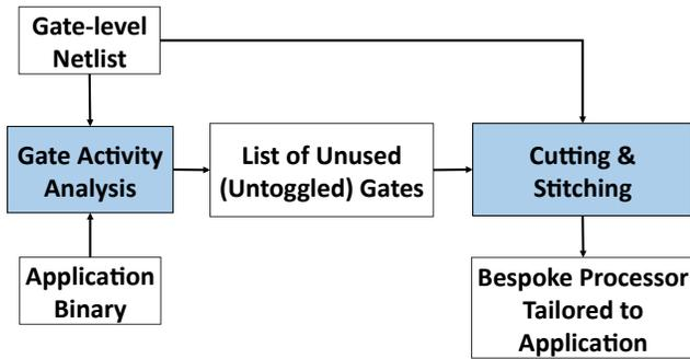
**Figure 5: Our technique performs input-independent gate activity analysis to determine which gates of a processor cannot be toggled in any execution of the application. These gates are then cut from the design to form a custom, bespoke processor with reduced area and power.**
