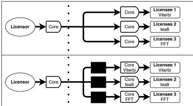
**Figure 1: General purpose processors are overdesigned for a specific application (top). A bespoke processor design methodology allows a microprocessor IP licensor or licensee to target different applications efficiently without additional software or hardware development cost (bottom).**
