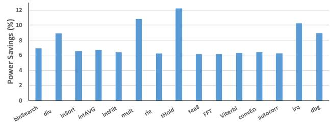
**Figure 15: Power savings achieved by oracular power gating with no overheads are significantly lower than those achieved by bespoke processors for the same applications, even when each module is allowed a separate power domain and a wake-up latency of 0 is assumed.**
