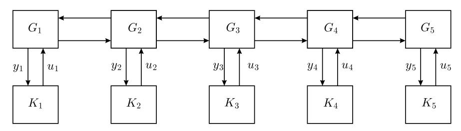
Control design problem is to find K which is block diagonal, whose diagonal blocks are 5 separate controllers.
