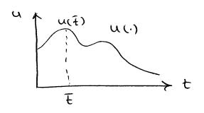
Controllability given a state, can we find input to bring the state to given state at a given time.
