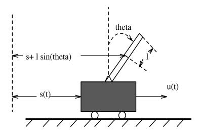
Figure 1: Inverted pendulum on a cart.
