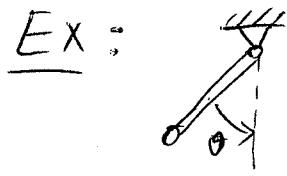
$$\begin{aligned}\dot{\theta}_1 &= \dot{\theta}_2 \\ \dot{\theta}_2 &= -a \sin \theta_1 - b \theta_2\end{aligned}$$
