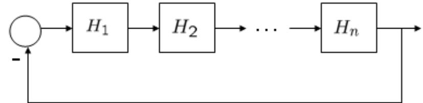
TYSON & OTHMER, THRON:  $H_i(s) = \frac{b_i}{s + a_i}$ ,  $\gamma_i := \frac{b_i}{a_i}$
