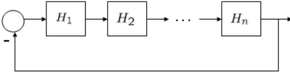
$$\begin{aligned}\dot{\psi}_1 &= -f_1(\psi_1) - g_n(\psi_n) \\ \dot{\psi}_2 &= -f_2(\psi_2) + g_1(\psi_1) \\ &\vdots \\ \dot{\psi}_n &= -f_n(\psi_n) + g_{n-1}(\psi_{n-1})\end{aligned}$$
