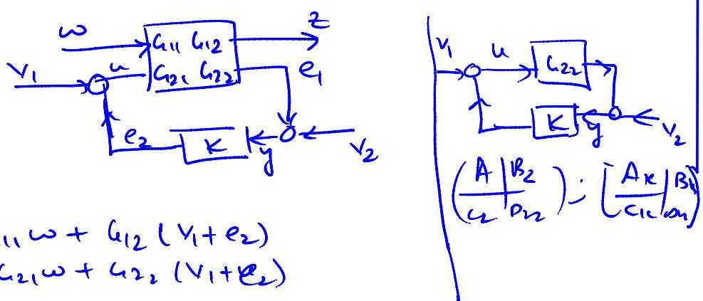
$$z = G_{11}\omega + G_{12}(v_1 + e_2)$$
