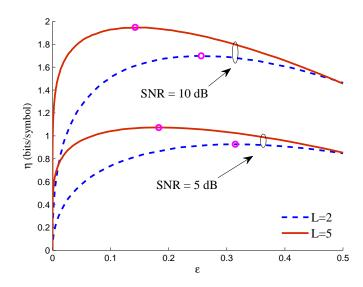
Fig. 1. Gooput  $\eta$  (bits/symbol) vs. PHY outage probability  $\varepsilon$  for  $L=2,5,~{\rm SNR}=10~{\rm dB}$
