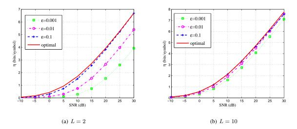
Fig. 4.  $\eta$  (bits/symbol) vs. SNR (dB), for  $\varepsilon=0.001, 0.01, 0.1,$  and  $\varepsilon^{\star}$
