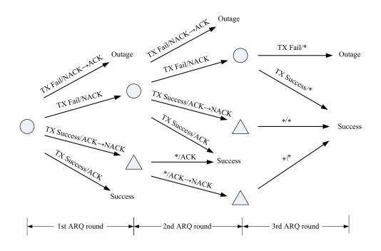
Fig. 7. The ARQ process with non-ideal feedback with an end-to-end delay constraint d = 3.
