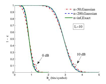
Fig. 5. Success probability  $1 - \varepsilon$  vs. transmitted rate  $R_{\varepsilon}$  (bits/symbol) for  $n = 50, 200, \infty, L = 10$  at SNR = 0 and 10 dB
