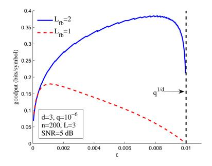
Fig. 9. Goodput  $\eta$  (bits/symbol) vs. PHY outage probability  $\varepsilon$  with  $L_{\rm fb} = 1$  and 2 in Rayleigh fading feedback channel for SNR = 5 dB, n = 200, L = 3, d = 3 and  $q = 10^{-6}$ .
