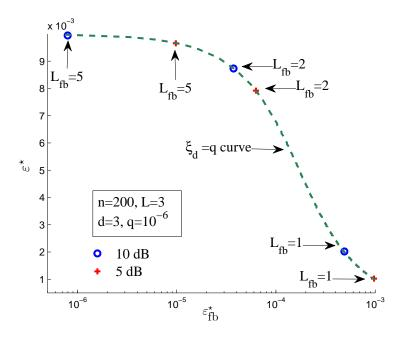
Fig. 8.  $(\varepsilon^*, \varepsilon^*_{\rm fb})$  with  $L_{\rm fb} = 1, 2$  and 5 in Rayleigh fading feedback channel for  $n = 200, d = 3, q = 10^{-6}$ , and L = 3 at SNR = 5 and 10 dB. The curve specifying the  $(\varepsilon, \varepsilon_{\rm fb})$  pairs that achieve the reliability constraint  $\xi_d = q$  is also plotted.
