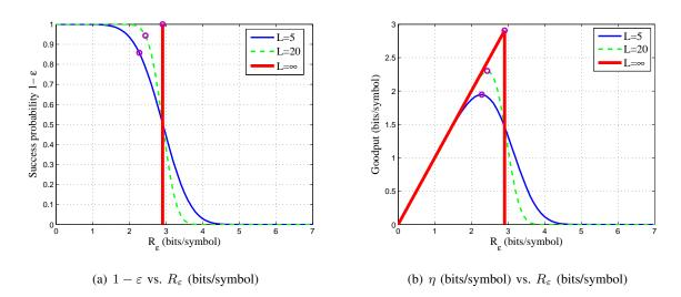
Fig. 3. Success probability  $1 - \varepsilon$  and  $\eta$  (bits/symbol) vs.  $R_{\varepsilon}$  (bits/symbol) for SNR = 10 dB
