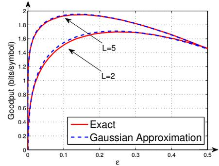
Fig. 1: Goodput (bits/symbol) vs.  $\varepsilon$ ,  $L = 2, 5$ ,  $\text{SNR} = 10$  dB
