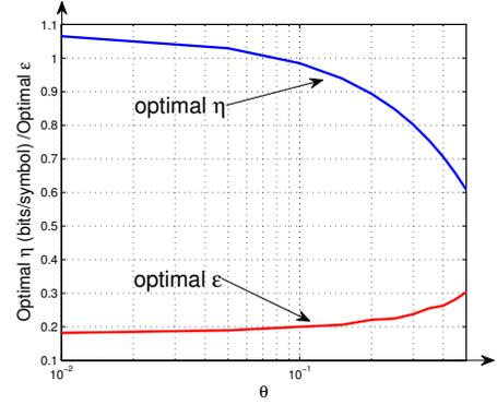
Fig. 5:  $\eta(\varepsilon^*)$  (bits/symbol) and  $\varepsilon^*$  vs.  $\theta$ ,  $L = 5$ ,  $\text{SNR} = 5$  dB
