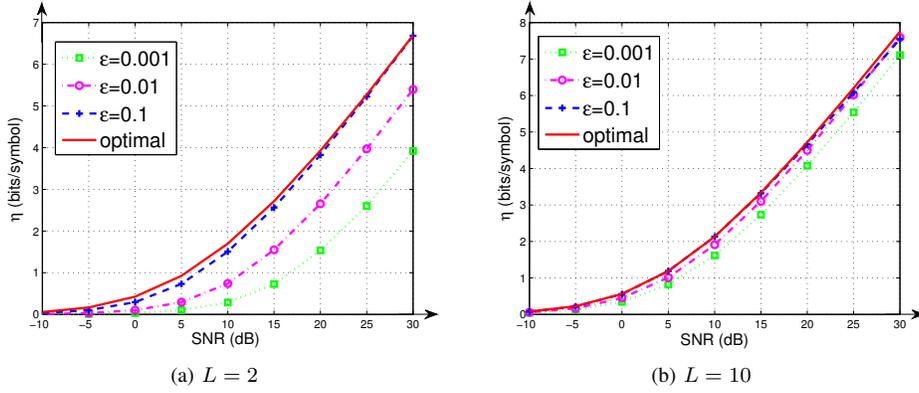
Fig. 4:  $\eta$  (bits/symbol) vs. SNR (dB),  $\varepsilon = 0.001, 0.01, 0.1$ , and  $\varepsilon^*$
