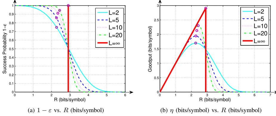
Fig. 3: Success probability  $1 - \varepsilon$  and  $\eta$  (bits/symbol) vs.  $R$  (bits/symbol), SNR = 10 dB
