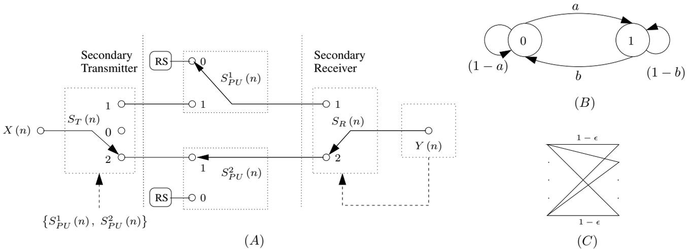
Fig. 2: Part (A) illustrates the system model. RS denotes a random source. At the time instant considered, we have  $S_{PU}^1(n) = 0$ ,  $S_{PU}^2(n) = 1$ ,  $S_T(n) = 2$  and  $S_R(n) = 2$ . Part (B) shows the Markov chain for the primary user occupancies  $S_{PU}^1(n)$  and  $S_{PU}^2(n)$  in the two channels. Part (C) is the  $Q$ -ary symmetric channel.
