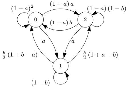
Fig. 3: Equivalent Markov chain for the transmitter state  $S_T(n)$  for the preference strategy of Section IV-A.
