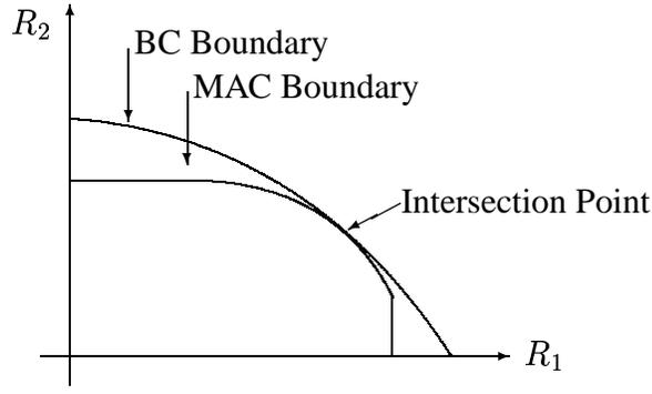
Figure 4: Capacity regions for the dual fading MAC and BC
