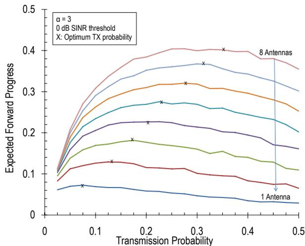
Fig. 8. Expected forward progress vs. transmission probability ( $p$ ) for  $n_R$  ranging from 1 (bottom) to 8 (top), for  $\alpha = 3$ ,  $\beta = 0$  dB, and no noise. The optimizing values of  $p$  are denoted with an X.
