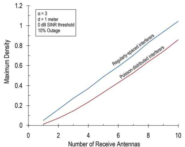
Fig. 9. The optimal density for both Regular and Poisson networks increases linearly with  $n_R$ , which regular networks having a slightly higher achievable density since nearby (dominant) interferers do not exist.
