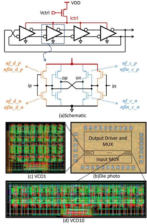
Fig. 3: VCO design example (a) Schematic of the VCO (b) Die photo of the fabricated chip (c) Layout illustration of VCO 1 (d) Layout illustration of VCO 10
