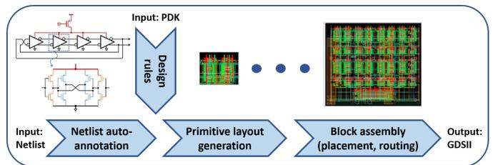
Fig. 2: Overview of the ALIGN layout generation process [12]
