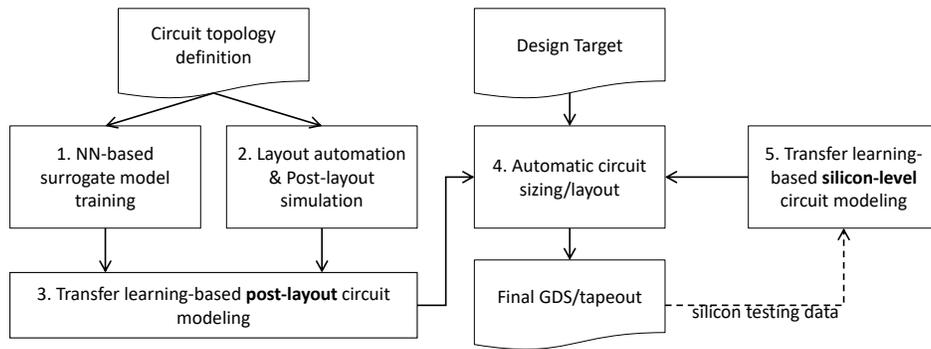
Fig. 1: Proposed design flow from specification to silicon
