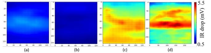
**Figure 13:** Instance-level IR drop heatmaps for (a) AES, (b) Dynamic\_node, (c) Ibex, and (d) JPEG in GF 12nm technology.
