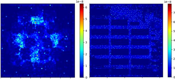
**Figure 8:** Example CMs ( $A/\mu m^2$ ) in “Set 1” (left) and “Set 2”(right) on a 45nm technology node.
