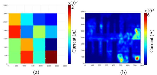
**Figure 1:** Current maps of (a) IBM power grid benchmark with uniform currents per region. (b) a RISC-V core.
