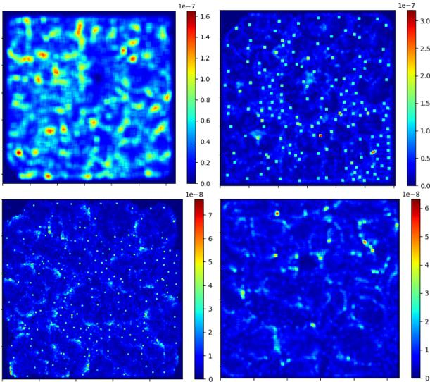
**Figure 9:** CMs of JPEG design from “Set 1” across four pdks ASAP 7nm (top-left), GF 12nm (top-right), FreePDK45 with Nangate Open Cell library (bottom-left), SkyWater 130nm(HD) (bottom-right)
