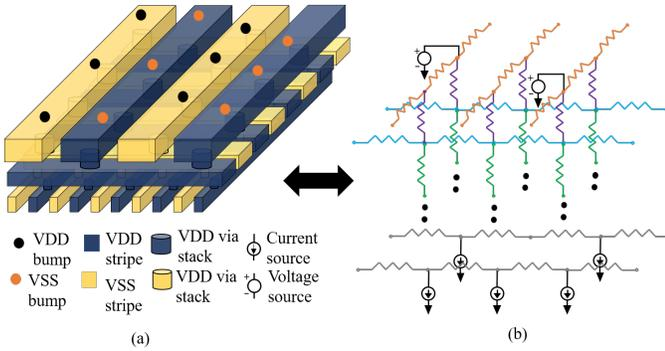
**Figure 2:** (a) A multilayer PDN stack and (b) its circuit netlist model.
