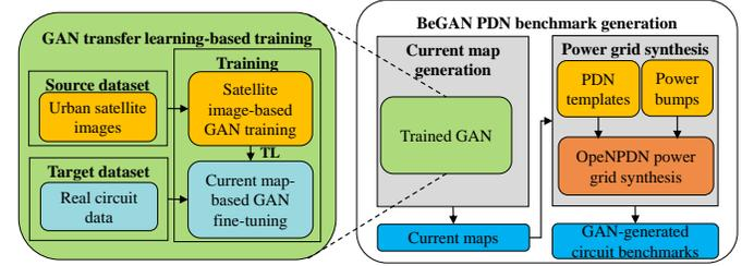
**Figure 3:** Overview of BeGAN benchmark generation: GANs are trained using TL to generate current maps. PDNs and power pad locations are generated using OpeNPDN [20].
