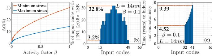
**Fig. 6.** Aging effects on 6-bit IDAC. Aging can (a) increase gain errors, (b) increase INL, (c) induce non-monotonicity.
