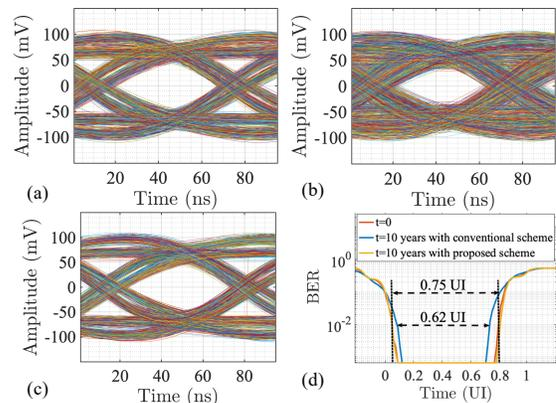
**Fig. 9.** Aging effects on eye diagram of HSLs: (a) at  $t = 0$ , (b) at  $t = 10$  years with the conventional scheme, (c) at  $t = 10$  years with the proposed scheme, (d) bathtub curve comparison in unit interval (UI).
