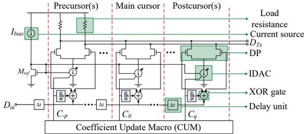
**Fig. 3.** Schematic of a feed-forward equalizer (FFE) architecture.
