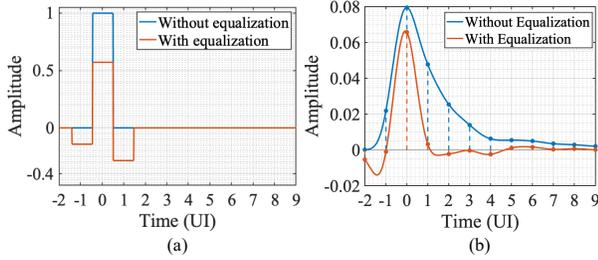
**Fig. 2.** An unequalized pulse with its precursor and postcursor, and its equalized output. The signal is sampled at integer multiples of the unit interval (UI), and the equalized signal provides low ISI at  $t \leq -1$  and  $t \geq 1$ .
