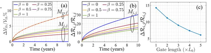
**Fig. 5.** (a)  $V_{th}$  degradation of  $M_{ref}$  and  $M_{i,j}$  due to aging with varying  $\beta$ . (b) Change in transfer ratio of  $M_{i,j}$  due to aging with varying  $\beta$ . (c) Change in transfer ratio of  $M_{i,j}$  with varying gate length,  $L$ .
