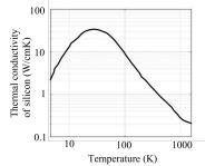
Fig. 5. Thermal conductivity of silicon as a function of temperature [12]. conductivity of silicon, which is an excellent heat conductor at room temperature, approaches that of an insulator [12].
