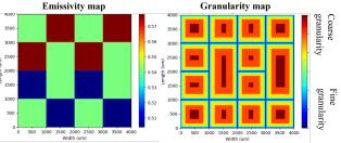
Fig. 7. Adaptive gridding strategy which maintains a high resolution (small element sizes) in the die regions with emissivity gradients. The testcase from [13] with four different element sizes.
