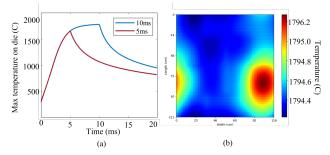
Fig. 9. (a) Maximum temperature on the die for two different pulse times for a 1800°C lamp and (b) temperature contours for the 10ms anneal pulse at time instance with the maximum temperature.
