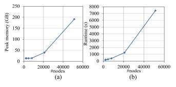
Fig. 10. Scalability analysis: (a) runtimes and (b) peak memory as a function of the number of nodes in the FDM simulation.
