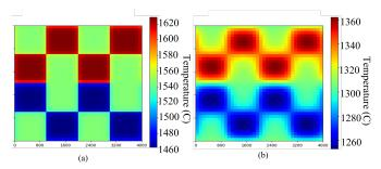
Fig. 6. Thermal profile of the testcase from [13] with a checkerboard pattern of emissivity (a) with and (b) without considering the dependence of the thermal conductivity of silicon on temperature. A lamp temperature of  $1800^{\circ}$ C and pule time of 5ms is used.
