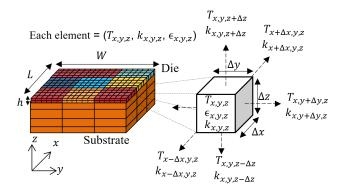
Fig. 4. FDM-based spatial derivative estimation.
