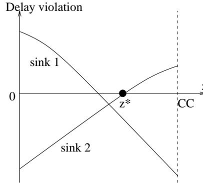
Figure 3: Delay violation function vs. Manhattan distance  $z$  of connection point.
