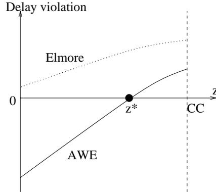
Figure 5: An example where using the Elmore delay and a higher order AWE delay may result in a different connection choice.
