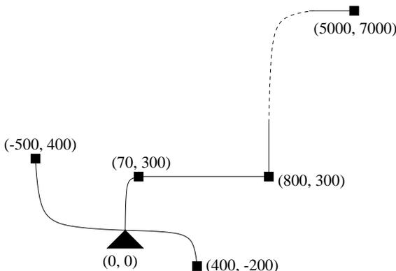
Figure 4: A routing tree on which Elmore delay gives large errors.
