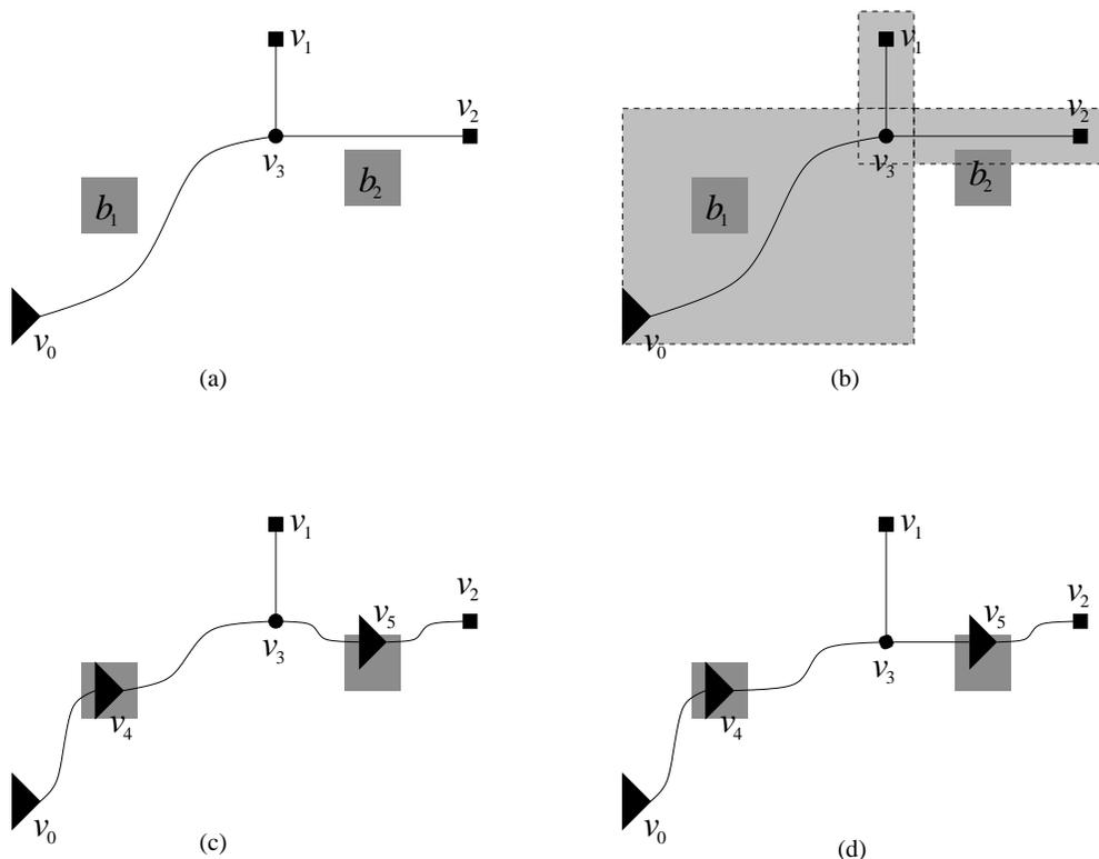
Figure 6: Buffer spaces, the territory box and their applications in buffer insertion.
