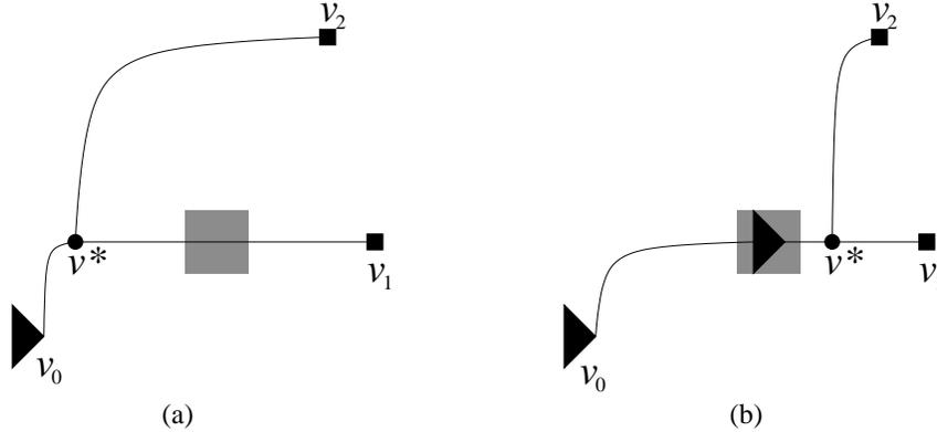
Figure 7: An example that buffer insertion can reduce wire cost further in non-Hanan optimization.
