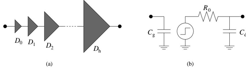
Figure 8: Cascaded drivers and driver model.
