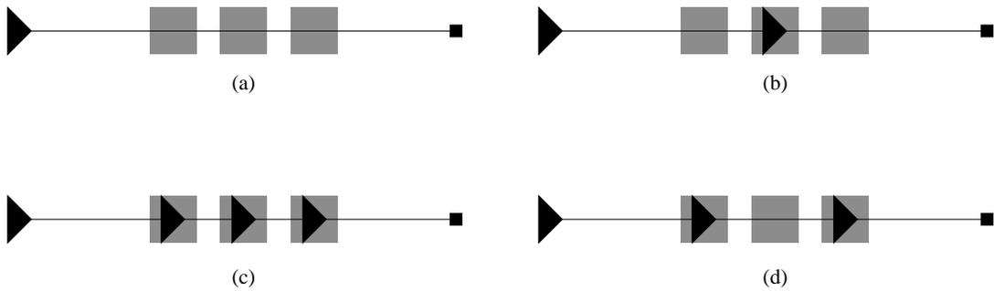
Figure 11: Iterative buffer insertion vs. iterative buffer deletion.
