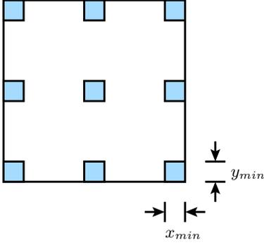
Fig. 3. The locations of the nine representative regions on the source plane. Each region has dimensions of  $x_{min} \times y_{min}$ . One region is located at the center of the plane, one is at the mid-point of each edge, and one is at each corner. Similarly, we have nine representative regions on the field plane.
