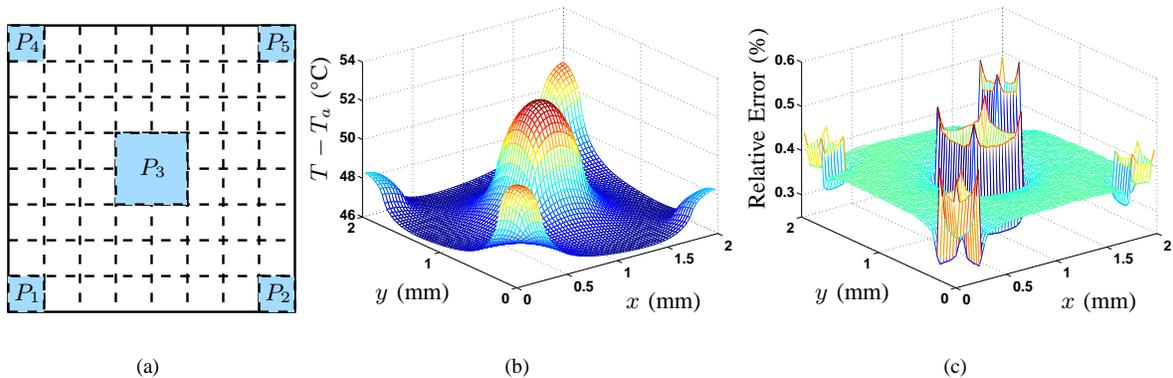
Fig. 8. Accuracy of Algorithm I (a) power source locations (b) computed temperature distribution above  $T_a$  using the proposed algorithm (c) relative error of the proposed algorithm compared with the result from a commercial CFD software package.
