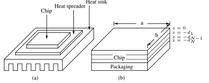
Fig. 1. Schematic of a VLSI chip with packaging (a) IC chip and the packaging structure (b) simplified model of the chip and packaging.
