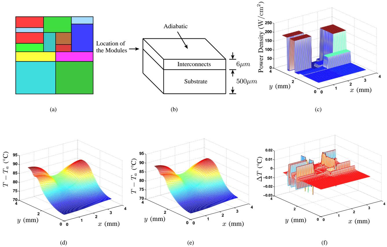
Fig. 10. Power and temperature distribution of a realistic chip (a) floorplan (b) schematic of the substrate and interconnect layers (c) power distribution (d) temperature distribution obtained using Algorithm I (e) temperature distribution obtained using Algorithm II (f) difference in the temperature distribution map obtained using the two algorithms.
