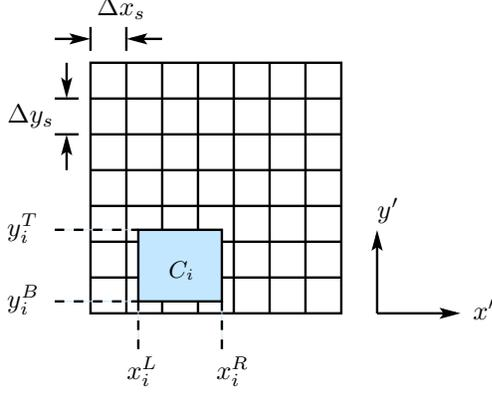
Fig. 5. Calculating the power density map from the given layout geometries and the power generated by each circuit component.
