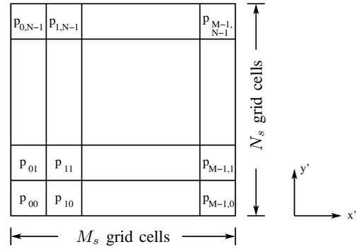
Fig. 4. The arrangement of the  $M_s \times N_s$  grid cells on the source plane.
