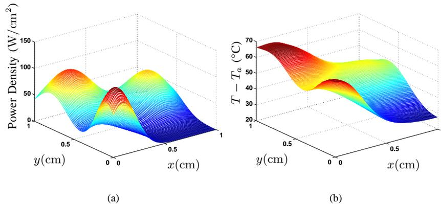
Fig. 11. Cell level power density and temperature distribution of a 1cm×1cm chip (a) power density distribution (b) temperature distribution.
