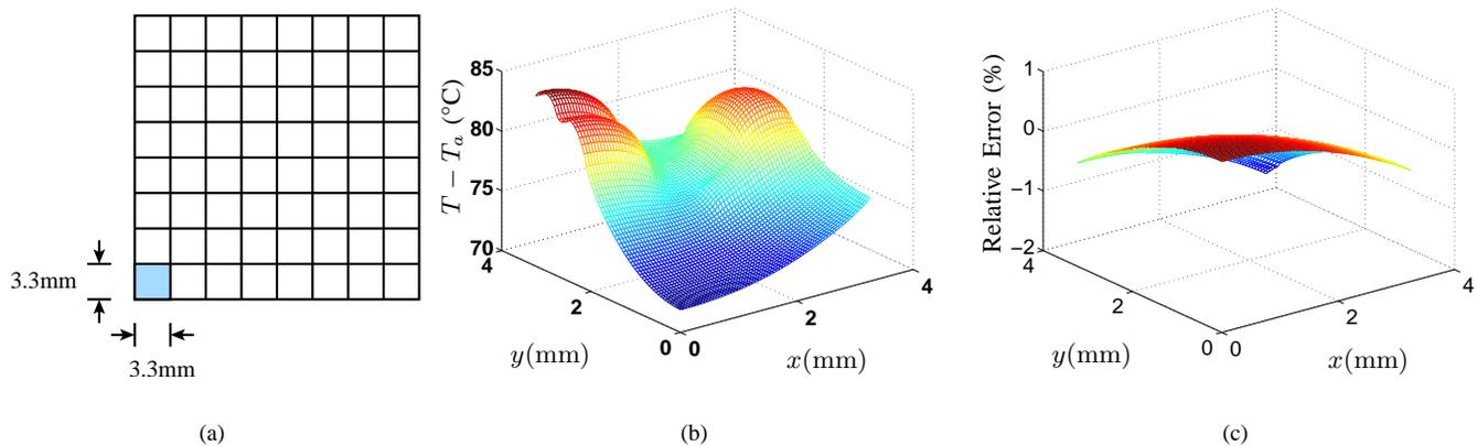
Fig. 12. Effectiveness of Algorithm III (a) location of the coarse grid cell  $CGC(0,0)$  that has higher requirement on thermal simulation (b) temperature map within  $CGC(0,0)$  calculated using Algorithm III (c) relative error of Algorithm III compared with Algorithm II applied with a fine grid over the entire chip.
