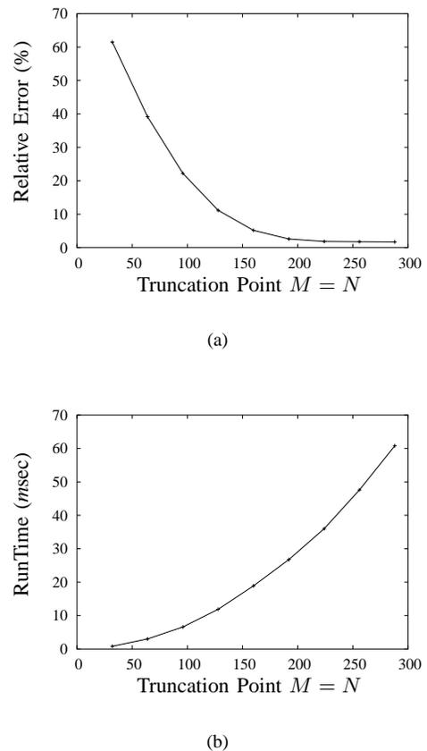
Fig. 9. Accuracy and computation time of the direct application of the Green function method (a) relative error in  $T - T_a$  versus truncation point (b) runtime versus truncation point.
