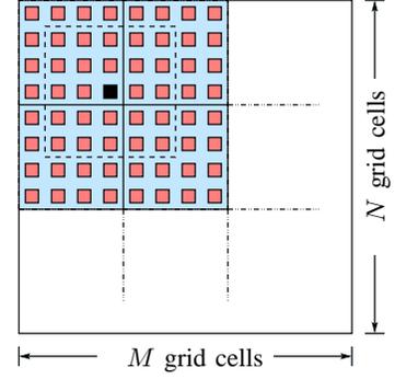
Fig. 7. A mixed signal chip where the analog block has higher requirement on the accuracy of thermal simulations. The logic gates and analog functional units within the dashed line constitute the set  $C(A)$ .
