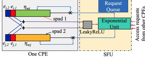
Fig. 8. Data flow corresponding to computation of an edge.
