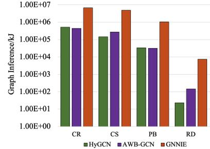
Fig. 16. Energy efficiency: GNNIE vs. HyGCN, AWB-GCN.
