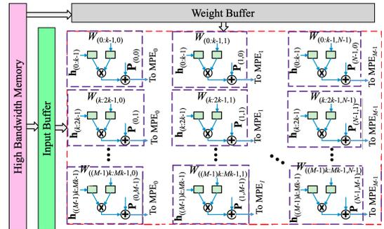
Fig. 4. Weight-stationary linear transformation of vertex features.
