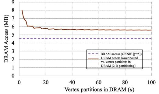
Fig. 17. Comparison of DRAM access of GNNIE with the lower bound on DRAM access vs vertex partitions in DRAM of 2-D graph partitioning.
