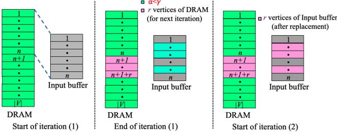
Fig. 10. Input buffer replacement policy during Aggregation.
