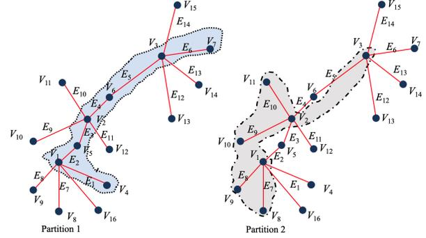
Fig. 9. Example illustrating the subgraph in the input buffer (left) and its evolution after cache replacement (right).
