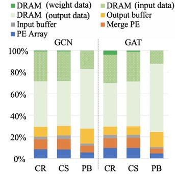
Fig. 15. Energy breakdown for GCN and GAT.
