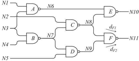
Fig. 5. An example circuit showing path reconvergence.
