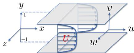
FIGURE 1. Geometry of a pressure-driven turbulent channel flow.
