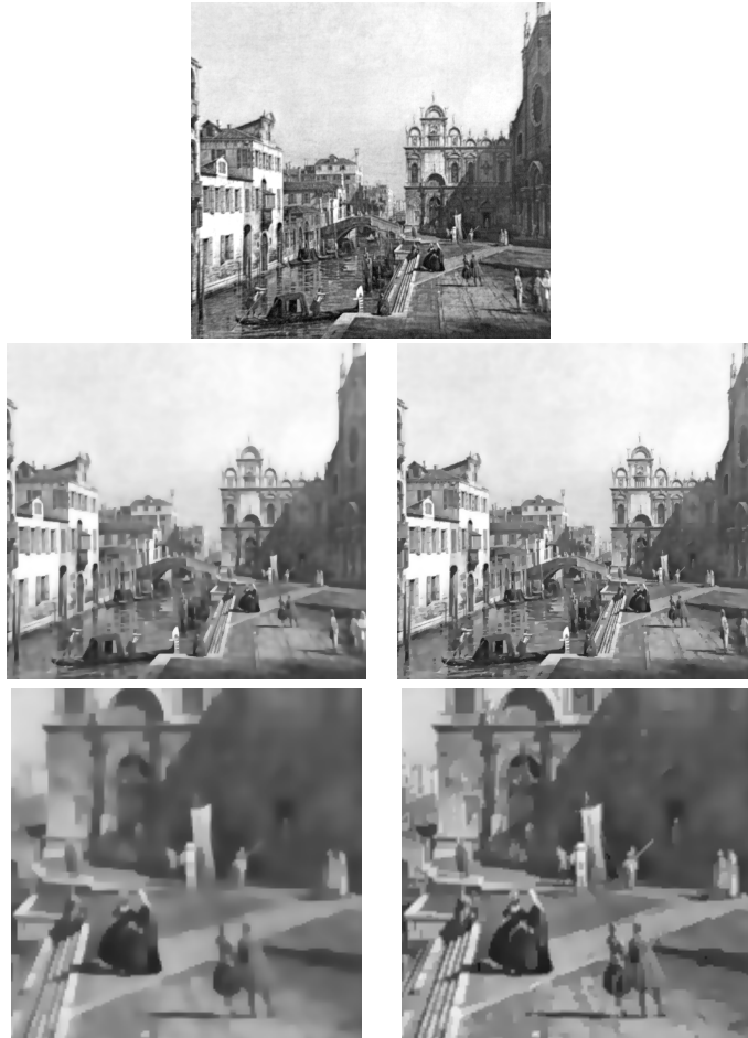
figure 4.9. Comparison of the Perona-Malik (Lorentzian) function (left) and the Tukey function (right) after 100 iterations. Top: original image. Middle: diffused images. Bottom: magnified regions of diffused images.
