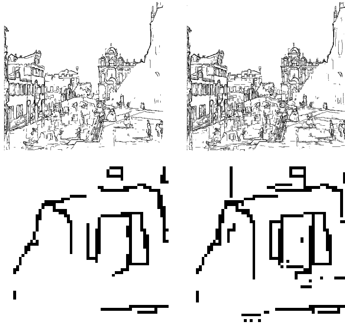
figure 4.16. Edges obtained with Perona-Malik (left); and Perona-Malik with additional spatial coherence in the line processes (right). Lower images show details on the gondola.
