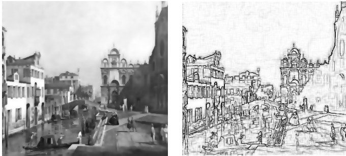
figure 4.15. Anisotropic diffusion with spatially coherent outliers. Left: smoothed image. Right: the value of the line process at each point taken to be the product, l_{s,h}l_{s,v} , of the horizontal and vertical line process at s .
