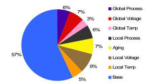
Figure 6: This figure breaks down the power consumption associated with worst case guardbands for various types of variations. If any source of variations can be tracked by SPDFT, the power associated with that guardband can be reduced under BTWC conditions.
