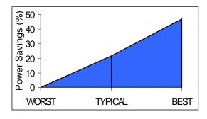
Figure 5: SPDFT can allow a processor that experiences BTWC variations to reduce power through supply voltage reduction. Additional power savings enabled by adapting to PVT variations can be up to 22% under typical case conditions and up to 47% in the best case if SPDTF allows adaptation to all sources of PVT variations.
