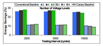
Figure 7: SPDFT in the context of a dynamic adaptation framework achieve up to 28% energy savings over a conventional worst case design and 12% energy savings over a canary circuit-based design. To make results more conservative, we do not account any overhead for canary circuits in the baseline design. Benefits are averaged over all benchmarks in our suite.
