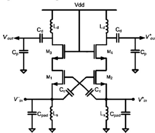
Fig. 5. Complete capacitor cross-coupled differential CGLNA stage.
