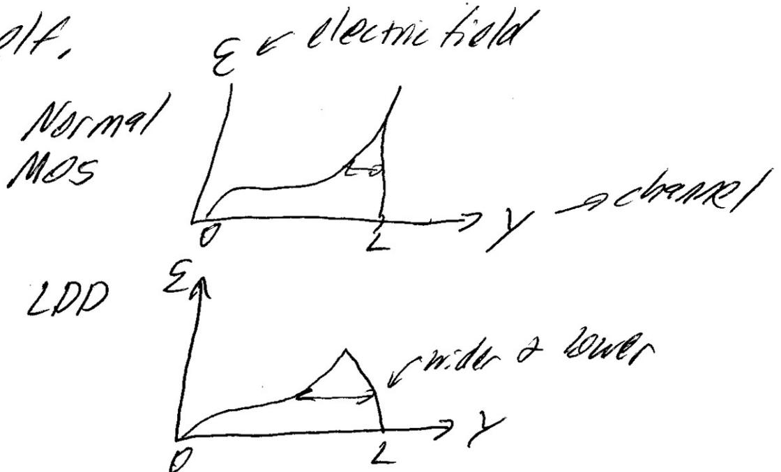
b.) The charge in the channel is  $\sim C_{ox}(V_g - V_t)$ . As  $V_g$  increases, the charge density increases and begins to exceed the level of n- in the lightly doped regions.
