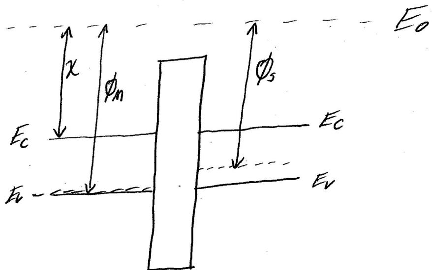
$$\begin{aligned} \phi_m &= \chi + E_c - E_f \\ &= \chi + E_c - E_v = \chi + E_g \\ &= 4.05 + 1.1 \text{ eV} = \underline{5.15 \text{ eV}} \end{aligned}$$
