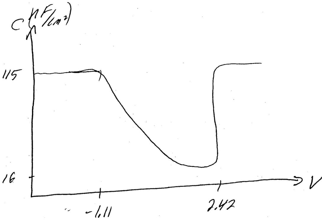
If  $n+p$  are switched, then  $\Delta\phi_{ns}$ ,  $2\phi_f$  &  $\Delta\phi_{ox}$  change signs.  $-\frac{Q_f}{C_f}$  stays constant. Also the voltages must change sign or we will forward bias the source-substrate & drain substrate junctions.
