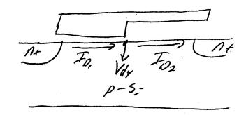
We will introduce an internative voltage, Vdy, as the voltage at the border between the two transistor halves.
