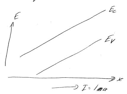
No Fermi Level is associated with this diagram because it is not in equilibrium, (There is an applied tield)
