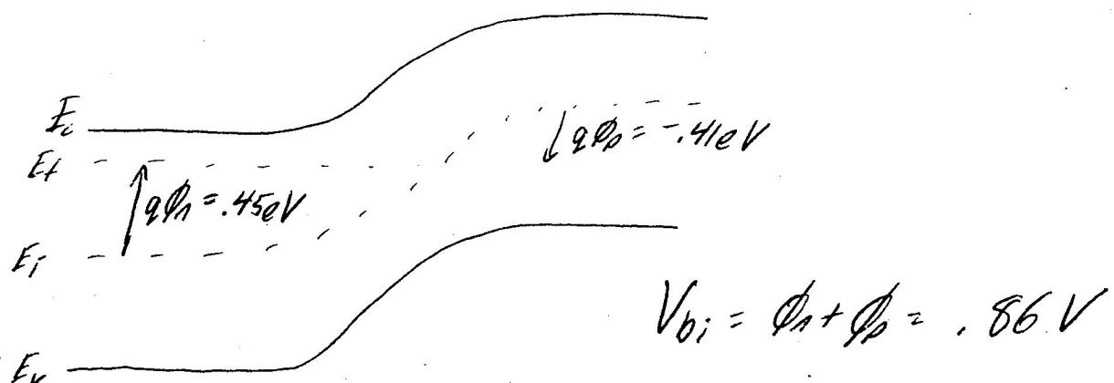
$$x_p = \sqrt{\frac{2e}{q} V_{bi} \frac{N_d}{N_a(N_a + N_d)}} = 0.11 \mu\text{m}$$
