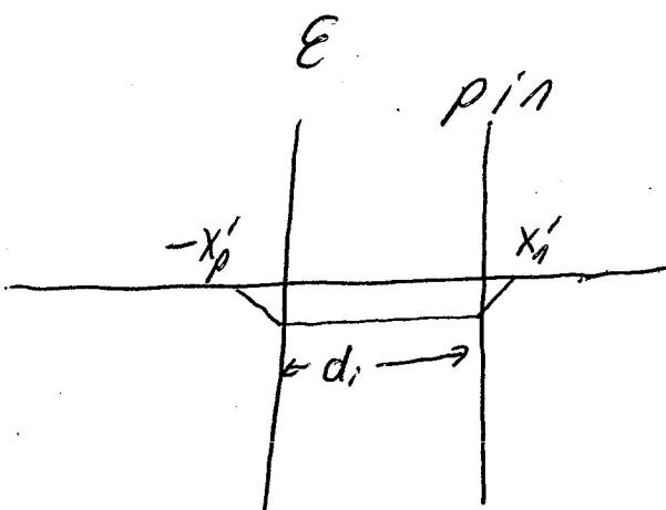
Since  $d_i$  is  $\gg x'_p, x'_n$  in the p-i-n diode and we know that the area of the E-field curve =  $V_{bi}$  ( $-\int E dx = V_{bi}$ )
