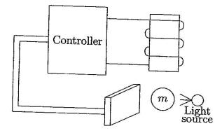
Figure 1.26: Magnetic suspension system of Exercise 1.18.
