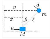
Figure 1: The inverted pendulum on a cart problem.
